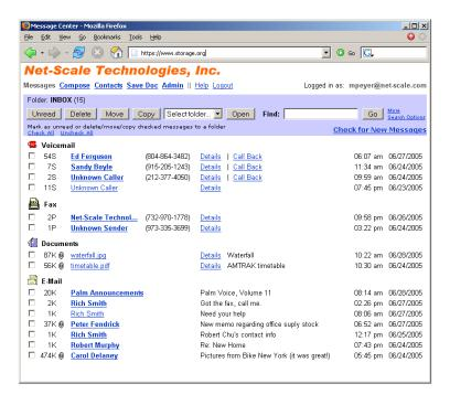
Figure 6: The web interface for listing of a directory which contains e-mail, voice mail, and fax messages in addition to regular files.
