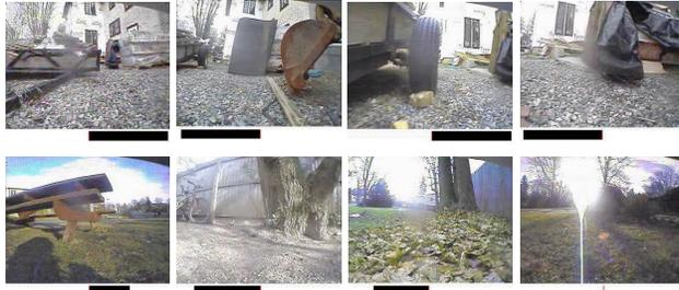
Figure 2: DAVE: Snapshots from the left camera while the robots drives itself through various environments. The black bar beneath each image indicates the steering angle produced by the system.
