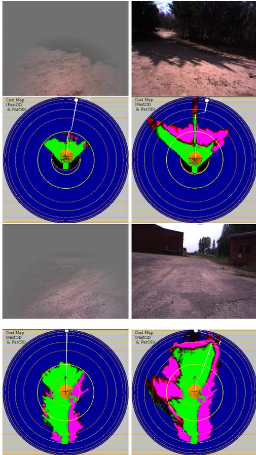
Figure 5: Net-Scale/NYU LAGR : H-Polar Map Two examples of Left: short range (stereo) obstacle map, and Right: the long range map. Above each example are the input images to the system. We overlay the images on the left with a grey fog which represents the distance to which the system can “see” using only the short-range stereo system. The online learning system on the right learns to classify the long-range obstacles in different environments.
