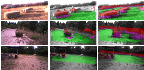
Figure 6: Net-Scale/NYU LAGR : Qualitative examples of the success of the long-range classifier in different terrain. **Left:** RGB input; **middle:** training labels; **right:** classifier output. Green is traversable, red is obstacle, and pink is foot-line. Notice that the classifier output in the far right column allows the navigation system to ‘see’ much further.
