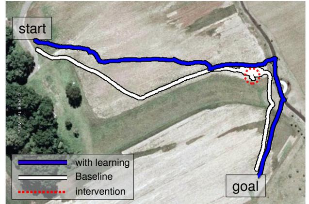
Figure 7: Net-Scale/NYU LAGR : Aerial plots of comparison runs of long-range and Baseline systems. This aerial view is approximately 300 meters wide. The long-range system in blue identified the large tall-grass area from the beginning and stays out of trouble while the Baseline system got close to the grass and got into trouble.
