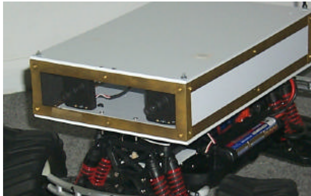
Figure 6. View of the Box housing the onboard sensory electronics.
